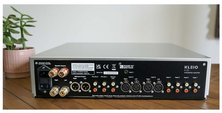
A raft of analogue connections spread over four RCA and two XLR inputs, with outputs shared over variable (XLR/RCA) and fixed (RCA). A 3.5mm jack will offer an optional digital input in future models
