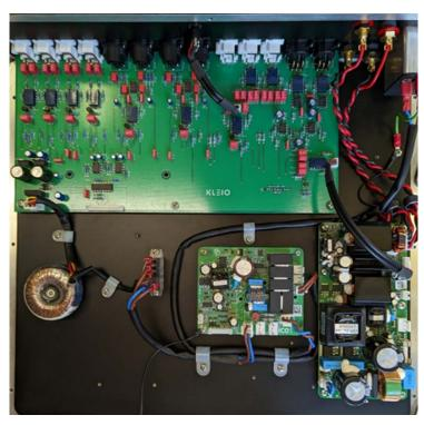
Short signal paths and clearly laid out internals within the K135, with its transformer given plenty of space. Digital module will live above the main PCB (top of image)
